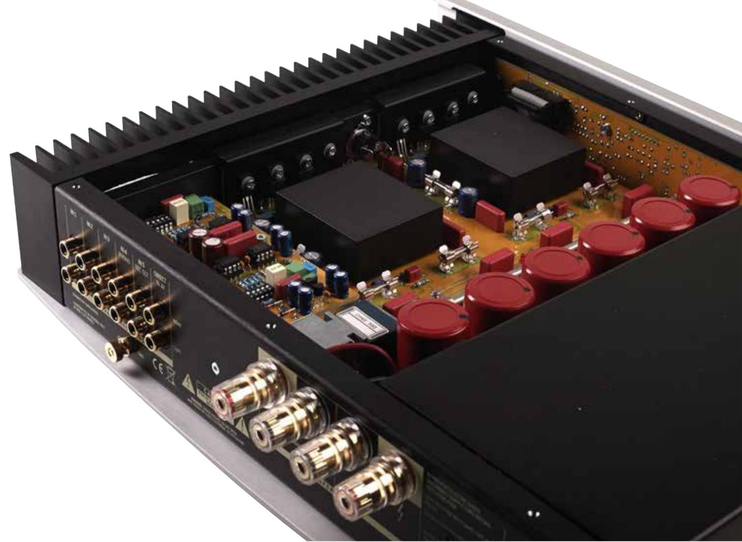
The amplifying section and the regulated power supply are housed in a single circuit board. This has almost entirely eliminated the internal wiring and kept the signal path as short as possible. Large areas of ground plane achieve optimum shielding and reduction of ground impedance. The amplification circuitry, fruit of long experience and intensive testing, is contained in two proprietary modules, completely realized with discrete components.
