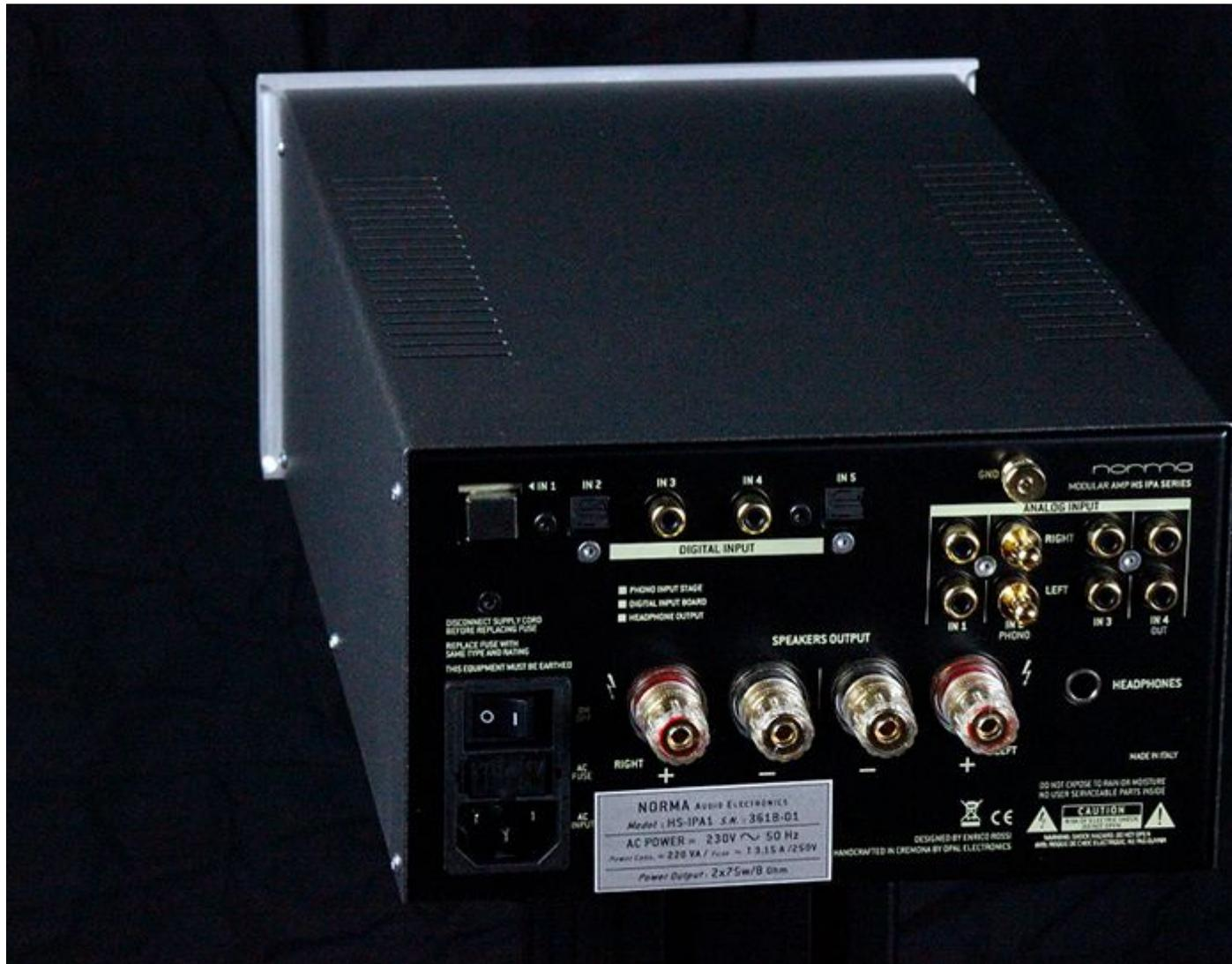
The connectors are all high quality and gold plated. There are four pairs of analogue RCA inputs, one pair of which connects to the optional phono stage, as well as USB, Toslink and S/PDIF for the optional DAC. The headphone socket is also on the rear panel - the matching amplifier is another optional extra. The Norma remote control is a chunky aluminium lump with a large array of buttons to cover every function. The buttons are a little small but it works perfectly well.
